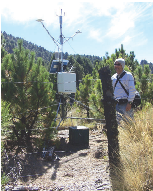
WebFigure 1. The Nevado de Colima automated weather station photographed on 15 Nov 2008. The barb wire was put in place by the Nevado de Colima National Park in 2001, shortly after the station was installed, and has been quite effective at protecting the sensors from cattle that graze freely in the area.
