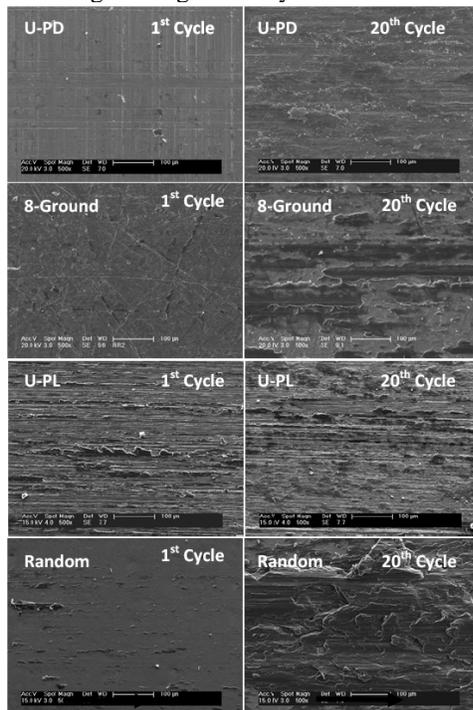
Fig. 2 SEM of different textured surfaces tested under dry conditions for 1<sup>st</sup> and 20<sup>th</sup> cycles. Arrows indicated the sliding direction of the pin relative to the plate.
