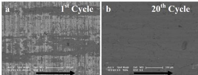
Fig. 2: Backscattered SEM of UPD surfaces tested under dry conditions for (a) 1<sup>st</sup> and (b) 20<sup>th</sup> cycles. Arrows indicated the sliding direction of the pin relative to the plate.
