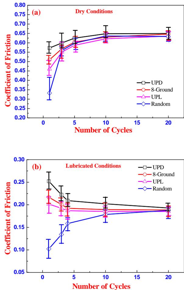
Fig. 1: Variation of average coefficient of friction with number of cycles for different surface textures under (a) dry and (b) lubricated conditions.
