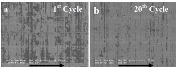
Fig. 3: Backscattered SEM of UPD surfaces tested under lubricated conditions for (a) 1<sup>st</sup> and (b) 20<sup>th</sup> cycles. Arrows indicated the sliding direction of the pin relative to the plate.
