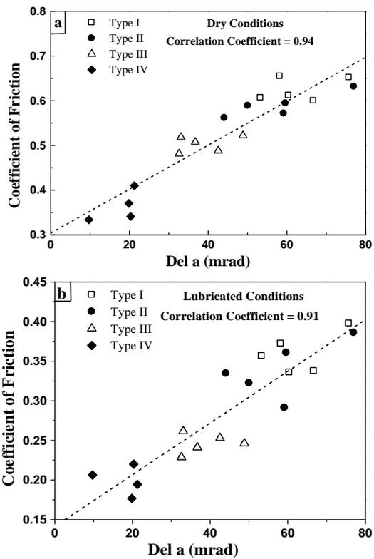
**Figure 8:** Variation of average coefficient of friction with roughness parameter, 'Del a' for various surface textures under dry and lubricated conditions.
