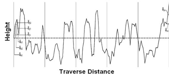
**Figure 7:** Calculating the mean slope of the profile.
