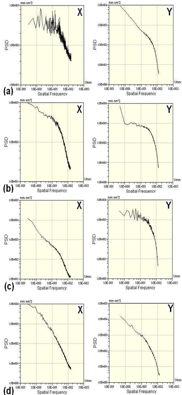
**Figure 2:** PSD Profiles of Types (a) I, (b) II, (c) III, and (d) IV surface textures.
