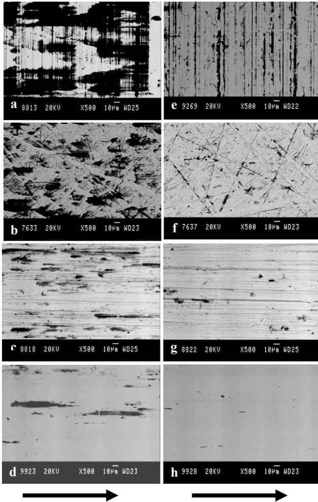
**Figure 5:** Backscattered scanning electron micrographs of steel plates for various surface textures after sliding tests under dry (a, b, c, d) and lubricated conditions (e, f, g, h) with (a, e) surface roughness of  $R_a = 0.19 \mu\text{m}$  (Type I), (b, f)  $R_a = 0.18 \mu\text{m}$  (Type II), (c, g)  $R_a = 0.14 \mu\text{m}$  (Type III), and (d, h)  $R_a = 0.17 \mu\text{m}$  (Type IV). The arrows indicate the sliding direction of the pin relative to the plate.
