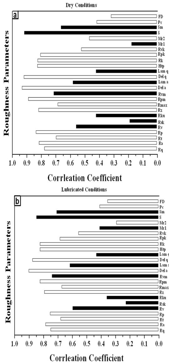
**Figure 6:** Correlation coefficient between coefficient of friction and roughness parameters under (a) dry and (b) lubricated conditions. White and dark bars represent positive and negative correlations, respectively.
