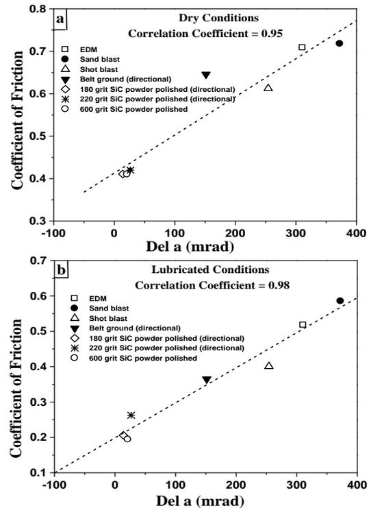
**Figure 11:** Variation of average coefficient of friction with roughness parameter ‘Del a’ for various surface textures under dry and lubricated conditions.
