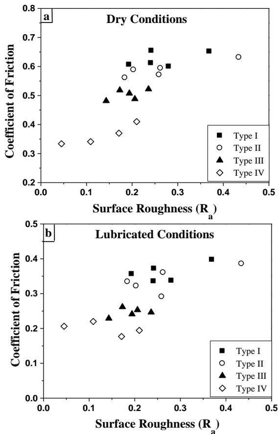
**Figure 3:** Variation of average coefficient of friction with surface roughness ( $R_a$ ) for various surface textures under (a) dry and (b) lubricated conditions.
