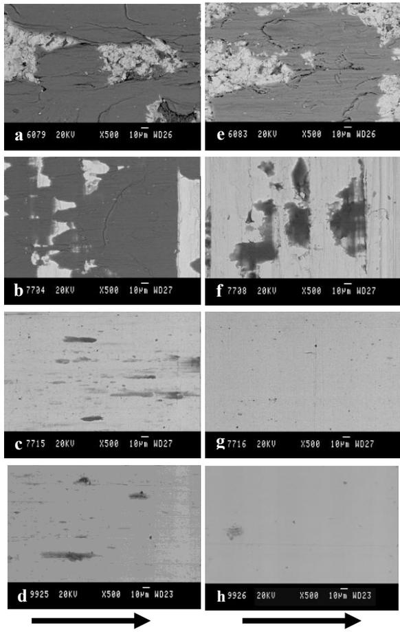
**Figure 12:** Backscattered scanning electron micrographs of steel plates for various surface textures after sliding tests under dry (a, b, c, d) and lubricated conditions (e, f, g, h) with (a, e) surface roughness of 'Del a' = 254 mrad (Type V), (b, f) 'Del a' = 151 mrad (Type VI), (c, g) 'Del a' = 26 mrad (Type VII), and (d, h) 'Del a' = 21 mrad (Type IV). The arrows indicate the sliding direction of the pin relative to the plate.
