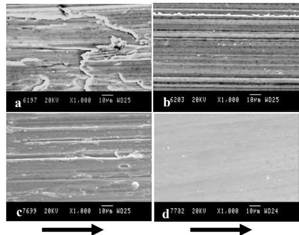
**Figure 13:** SEM micrographs of pin surface slid on steel plates under dry (a, b) and lubricated (c, d) conditions for Type V and Type VII surface texture with (a, c) 'Del a' = 254 mrad (Type V), and (b, f) 'Del a' = 26 mrad (Type VII). The arrows indicate the sliding direction of the plate relative to the pin.
