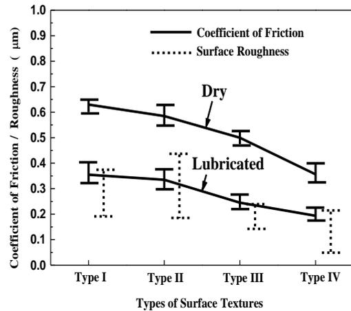
**Figure 4:** Variation of average coefficient of friction and surface roughness ( $R_a$ ) with surface texture.
